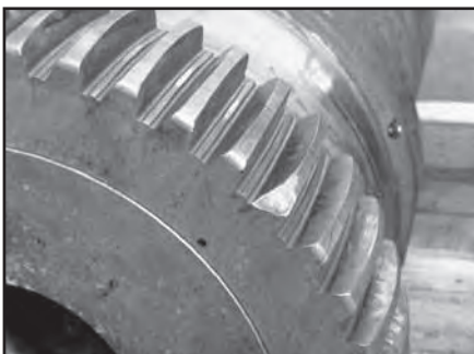
Tooth End Breakage due to over-misalignment
