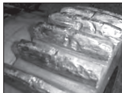
High speed cold mill with typical soap Molybdenum Disulfide after one year.
