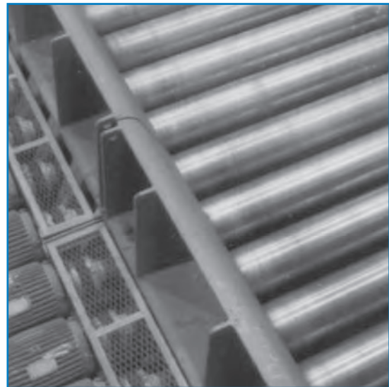
ELASTOMERIC™ Coupling for Runout table (shown under the guard) at a major hot strip steel mill
